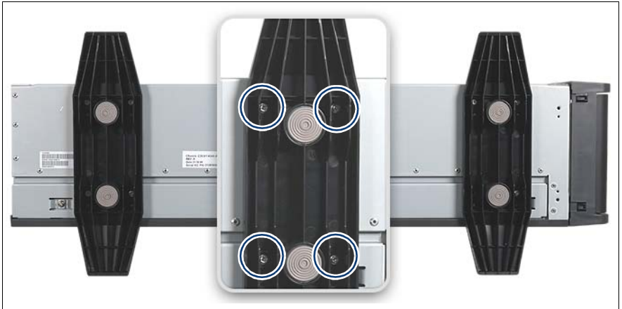
Figure 6: Removing the server feet
